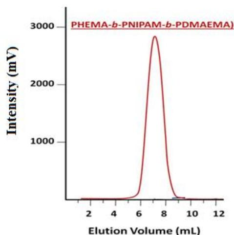
Figure 3- Gel permeation chromatogram of poly(HEMA-*b*-NIPAM-*b*-DMAEMA) triblock copolymer
