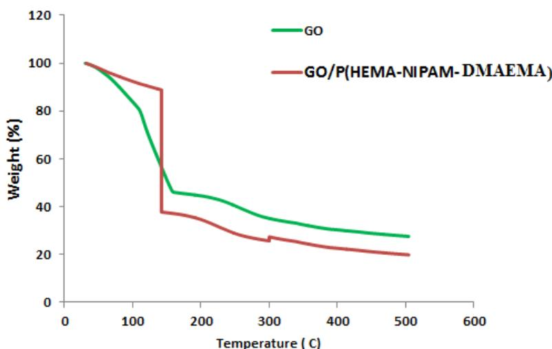
Figure 7- Thermo-gravimetry curve of GO and GO/poly(HEMA-*b*-NIPAM-*b*-DMAEMA) nanocomposite
