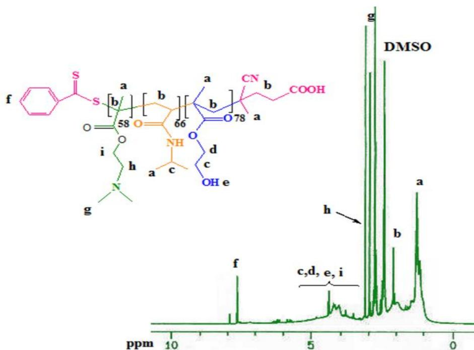
Figure 2-  $^1\text{H}$ NMR spectra of poly(HEMA-*b*-NIPAM-*b*-DMAEMA) triblock copolymer;  $^1\text{H}$ NMR spectra of PHEMA and PNIPAM were presented in our previous studies [31,32].
