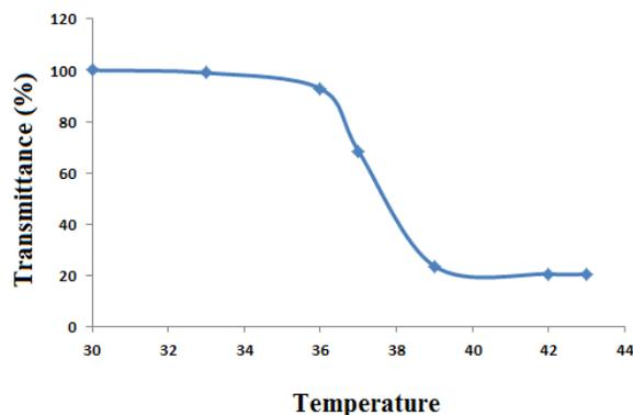
Figure 5- Low critical solution temperature of GO/poly(HEMA-*b*-NIPAM-*b*-DMAEMA) nanocomposite
