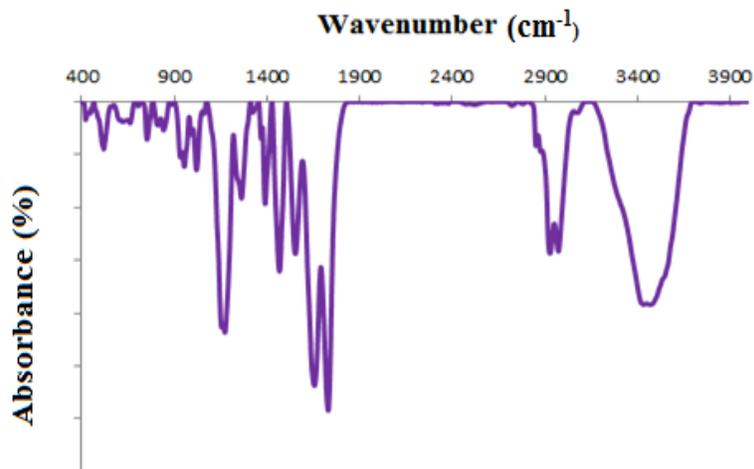
Figure 1- FT-IR spectra of poly(HEMA-*b*-NIPAM-*b*-DMAEMA) triblock copolymer; FT-IR spectra of PHEMA and PNIPAM were presented in our previous studies [31,32].
