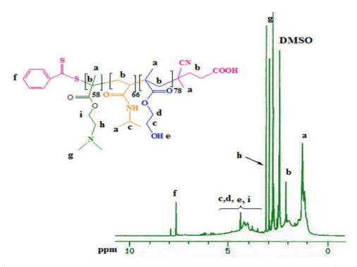
Figure 2- <sup>1</sup>HNMR spectra of poly(HEMA-*b*-NIPAM-*b*-DMAEMA) triblock copolymer; <sup>1</sup>HNMR spectra of PHEMA and PNIPAM were presented in our previous studies [31,32].
