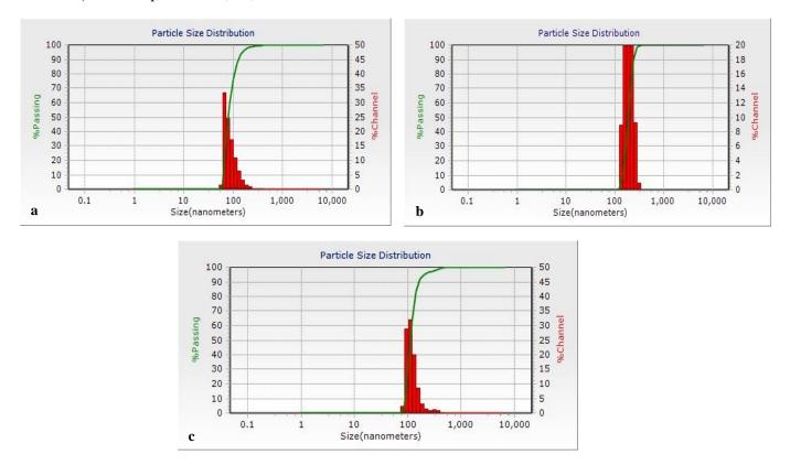
Figure 6- Dynamic light scattering of GO/poly(HEMA-*b*-NIPAM-*b*-DMAEMA) nanocomposite at a) 25 °C, b) 35 °C, and c) 42 °C
