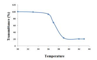
Figure 5- Low critical solution temperature of GO/poly(HEMA-b-NIPAM-b-DMAEMA) nanocomposite
