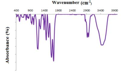
Figure 1- FT-IR spectra of poly(HEMA-b-NIPAM-b-DMAEMA) triblock copolymer; FT-IR spectra of PHEMA and PNIPAM were presented in our previous studies [31,32].
