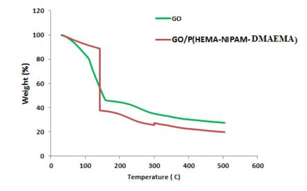
Figure 7- Thermo-gravimetry curve of GO and GO/poly(HEMA-b-NIPAM-b-DMAEMA) nanocomposite
